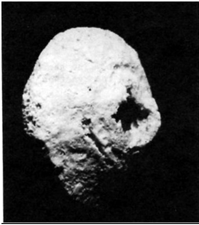
Fig. 6: Residual structure of corroded leaded bronze sheathing tacks, Lively (c. 1810), after digestion of tacks in warm 10 wt% nitric acid. The creamy-white solid was identified by XRD as cassiterite, \text{SnO}_2 . The chemical composition of the tack is listed in Table 1. Full width of image 6.6 mm.
